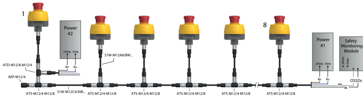
Figure 12. Option 1: Use a ATD-M12/8-M12/4 Connector in series with DCD device. If available, set the power supplies for parallel output.
